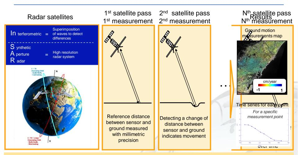
Ground movement is measured with radar satellites, comparing the distance between the sensor and the ground surface at different moments in time.
